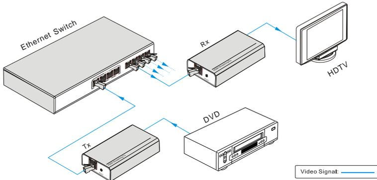
One or more receiver may be utilized in this case to broadcast signal from 1 transmitter to 1 or more receiver.
